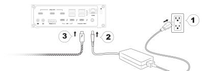
Connect the supplied Thunderbolt 5 cable to the port labelled [**Computer**] on the TS5 Plus.
