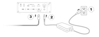
Connect the supplied Thunderbolt 5 cable to the port labelled [Computer] on the TS5.
