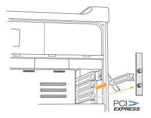
5 Hold the PCIe card fimrly by the ouside edge, push it into the slot making sure the PCI connectiins fit outside the computer.
