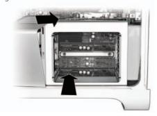
(b) (8 Core MacPro) Position the bottom front edge of the cover and then rotate the top back until the magnets snap it into place.
