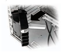
**3.5** Slide the CalDigit RAID Card into the PCI-Express slot Slide the CalDigit RAID Card into the PCI-Express slot. Make sure the card is fully seated.
