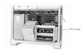
**1.23** Install any card(s) that you removed initially into their PCI- Express slots.
