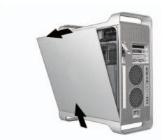
**Note:** To insure proper airflow (and avoid over heating), make sure that the fan module is running correctly and the side panel is completely closed. Place your hand near front of the Mac Pro and make sure that you can feel air moving.
