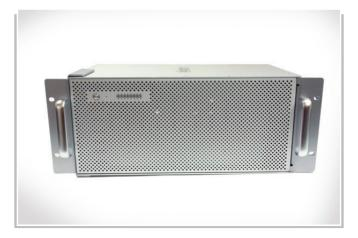
11. Using the Rackmount Rack Rail Mounting screws, you can now mount the HDPro on to the Rack rails.
