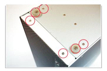
6. The HDPro Rackmount LOWER / RIGHT Kit and Type-II screws will be installed at this portion.
