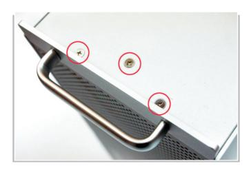
3. The top handle bar module will be replaced with the HDPro Rackmount UPPER / LEFT Kit AND Type-I screws.
