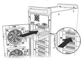
5. When the drive cannot be pushed in any further, push the drive-locking arm inwards until it clicks into place.
