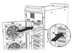
When the drive cannot be pushed in any further, push the drive-locking arm inwards until it clicks into place. 6. Top to bottom, use the same procedure to insert the remaining drives with drive number A0 being top, number A1 second down... all the way to number A7 at the bottom.
