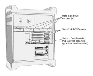
4. Always put the PCI card in Slot #3 or Slot #4 to obtain the optimal performance.
