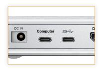
The other Type-C port is for device connection. It supports data transfer only and can provide up to 15W power to the device.
