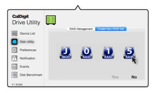
(5) Check all of the drives that you would like to include in the RAID set and select "create". Drives are numbered from top to bottom (A0 top, A1 A2 middle, A3 bottom).
