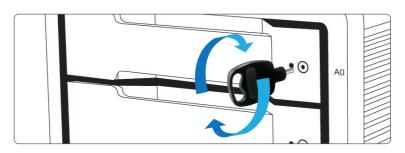
2 Insert the drive pin into the pin release until the handle of the drive module pops open.
