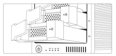
4 Insert the new drive in the same orientation as the drive you removed. The key holes should be on the same side as the drive labeling. Push the drive in all the way and then press in the drive module handle until it locks securely into place. Please do not use excessive force to insert the drive or you can damage it. The new drive will mount onto your OS.
