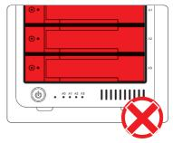
**6** To lock the new module into place, insert the drive key into the lock and turn counterclockwise.
