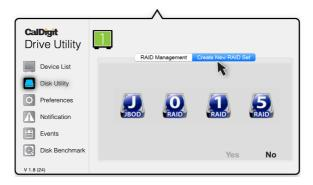
(5) Check all of the drives that you would like to include in the RAID set and select "create". Drives are numbered from top to bottom (A0 top, A1 A2 middle, A3 bottom).
