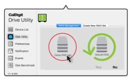
4 Go back into the "Disk Utility" tab and select "Create New RAID Set". Select the RAID mode you would like to create.
