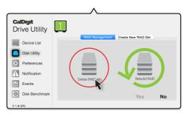
4 Go back into the "Disk Utility" tab and select "Create New RAID Set". Select the RAID mode you would like to create.
