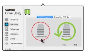
4 Go back into the "Disk Utility" tab and select "Create New RAID Set". Then Select RAID 5.
