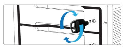
2 Insert the drive pin into the pin release until the handle of the drive module pops open.
